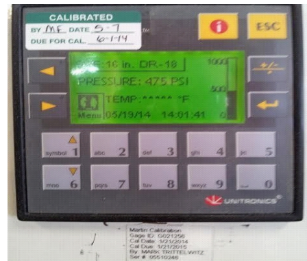
Hydro Test pressure gage and 5 second dwell period
