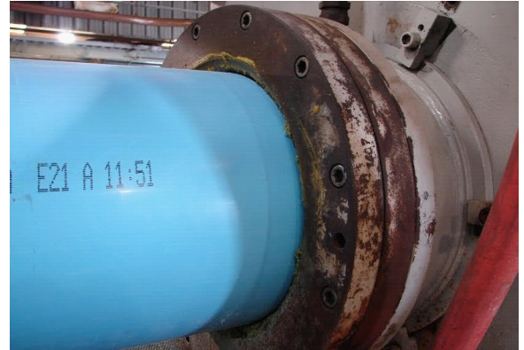
AWWA PVC Spigot inside gasketed Hydro Testing end cap
